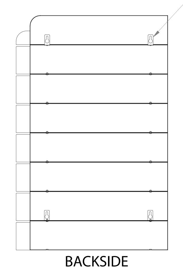
KEY-HOLE SLOT BRACKETS HOOK ONTO WALL SCREWS
